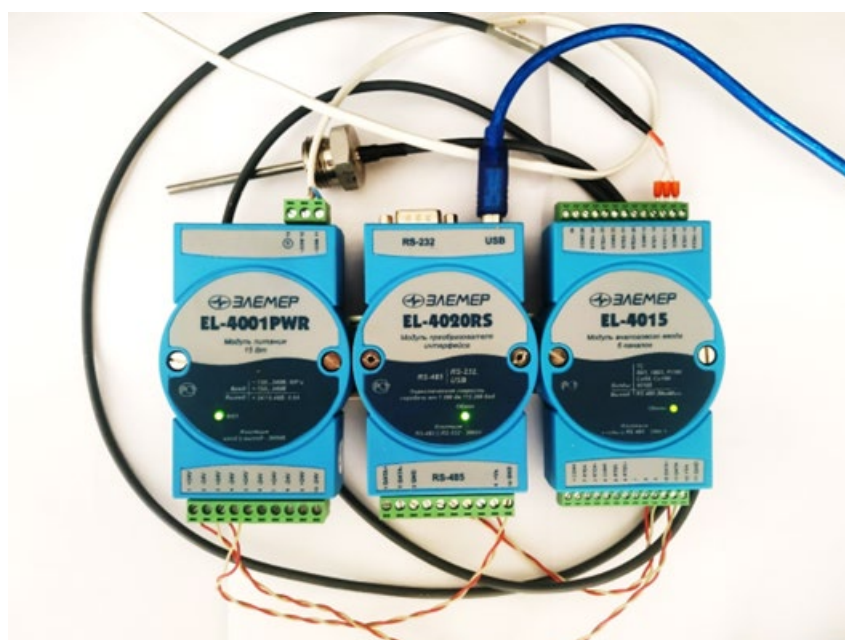
Figure 2. Assembled temperature control system
