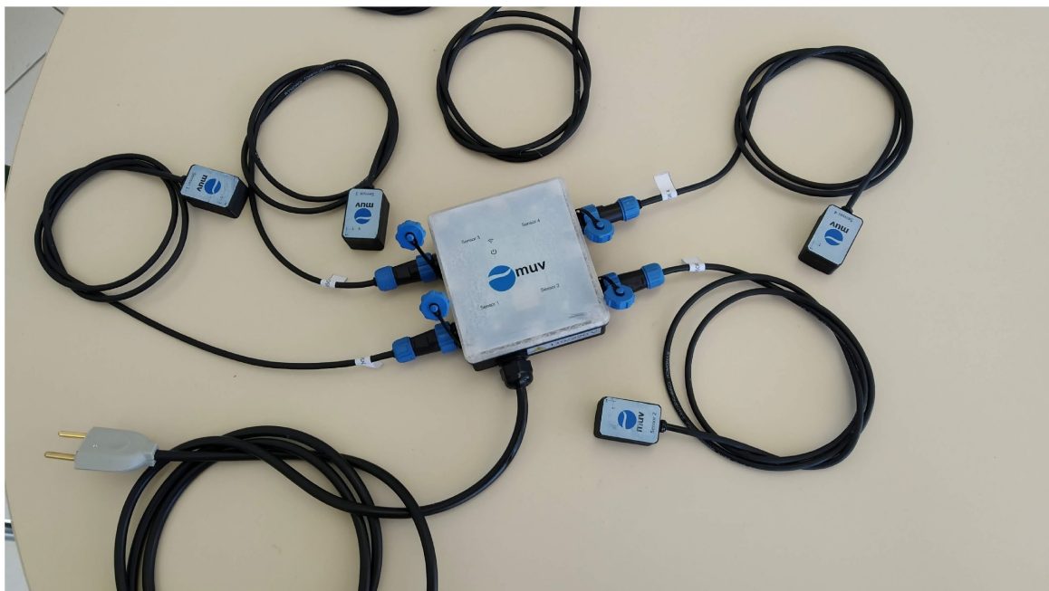
Figure 3. A vibration monitoring system composed of 4 sensors for simultaneously measuring 4 points in the same rotating machine
